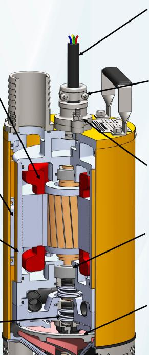
Power cables: Power cables are 100% water and oil proof available in any form PVC/EPR/HO7RNF depends upon the application where the pump is been used.
